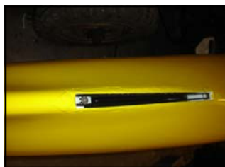
Gelcoat around finished skeg
