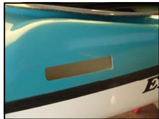
Glide box cut out on deck
