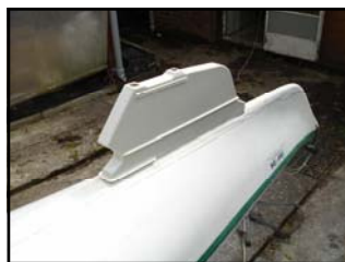
Skeg box positioned for marking out
