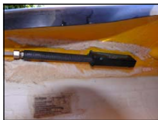
Glide tube fitted to glide box as seen from inside cockpit
