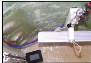
Routing of red and blue tubes from tiller block
