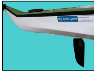
Skeg rudder blade deployed
