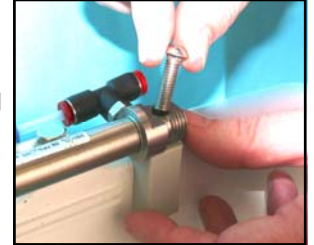
Attach ram to tapped block on top of skeg box.
