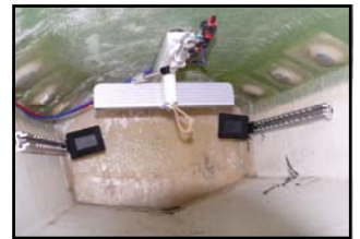
Example tiller block installation showing tiller pedal in relation to footpegs.
