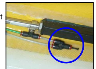
Blanking plug at glide box end
