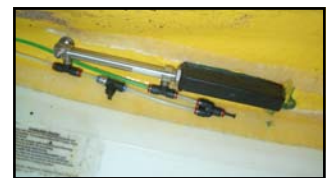
Glide cylinder inside cockpit
