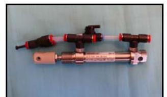
Rudder actuator ram assembly as supplied. The ram attaches to the top of the skeg box using the hole in the body of the ram, shown on the right in this image.
