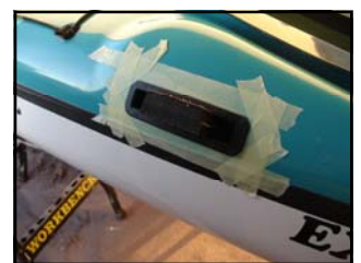
Glide box in place in deck
