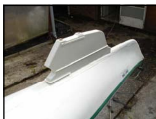
Skeg box positioned for marking out
