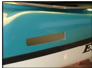
Glide box cut out on deck
