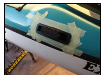
Glide box in place in deck
