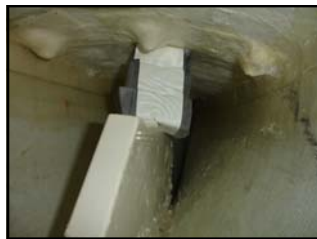
Skeg box wedged in hull with rubber blocks
